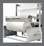
winding heavy GSM tubular fabrics used for FIBC applications where desired fabric tension can be adjusted by regulating torque through winder motor.
