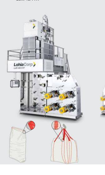
**Lofil** range of Spin-Draw-Wind Lines for polypropylene multifilament are compact and flexible machines designed to meet the value added yet dynamic requirements for varied applications.
