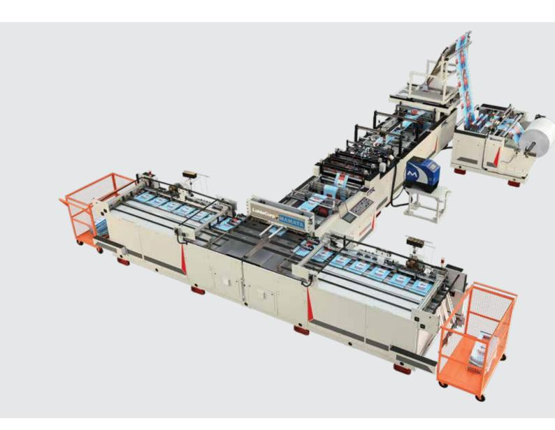
**LM-650** is the world's first high speed "Back Seam Sack" making machine from woven polypropylene tape fabric in flat form, laminated with reverse printed BOPP film, thereby giving a premium look for retail packaging. It is a compact machine equipped with integrated tubing and bag-making operations resulting in huge space savings.
