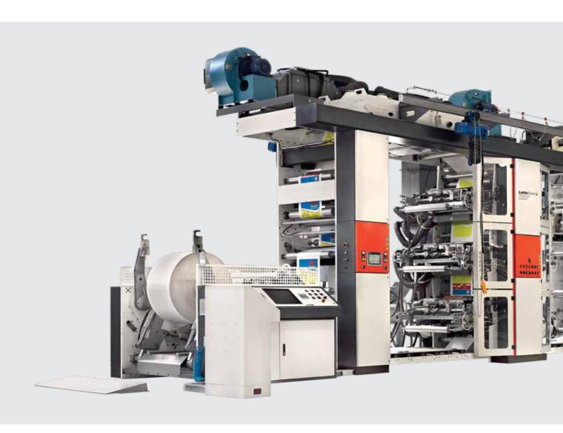
**Soloprint** is available in 4 or 6 colour options for tubular PP/HDPE woven fabric. Distinctively designed and precisely machined, equipped with new generation electronics, this machine maintains accuracy over a long and dependable life and ensures optimum performance. It includes both geared and gear-less types of machines.
